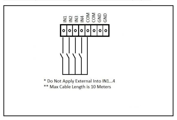
Only **volt-free** switches / sensors / relay outputs could be connected to GX2140 inputs.
